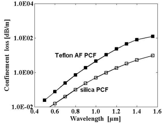
Figure 6: Confinement loss plot of conventional PCF with respect to wavelength with: 18 air holes,  $\Lambda=2.3\mu\text{m}$ ,  $d=1.38\mu\text{m}$  and  $d_1=d$ .
