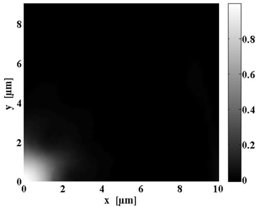
Figure 4: x-component of the electric field of the  $HE_{11}^x$  mode of the Teflon AF conventional PCF with: 18 air holes,  $\Lambda=2.3\mu\text{m}$  and  $d=d_1=1.38\mu\text{m}$ .
