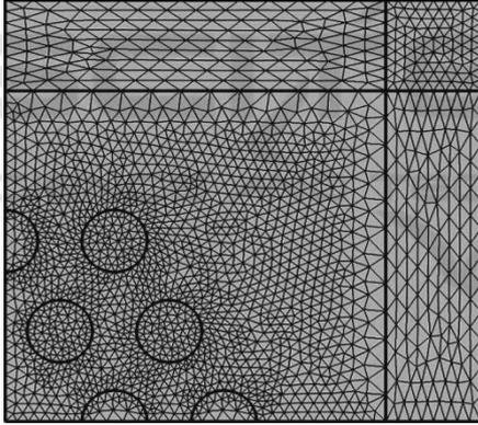
Figure 2: Computational window with meshing.
