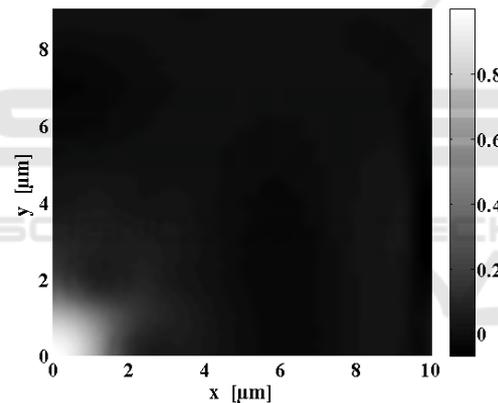
Figure 5: x-component of the electric field of the  $HE_{11}^x$  mode for the modified Teflon AF PCF with: 18 air holes,  $\Lambda=2.3\mu\text{m}$ ,  $d=1.38\mu\text{m}$  and  $d_1=0.92\mu\text{m}$ .
