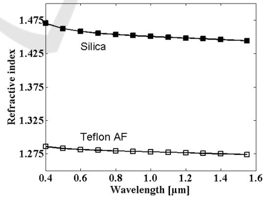
Figure 3: Material dispersion of silica and Teflon AF.
