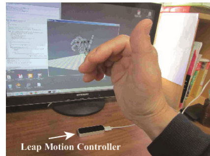
Figure 7: Digital hand system with LMC to get hand posture in real time.
