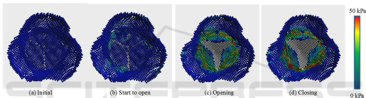
Figure 9: Stress distribution on the aortic valve.
