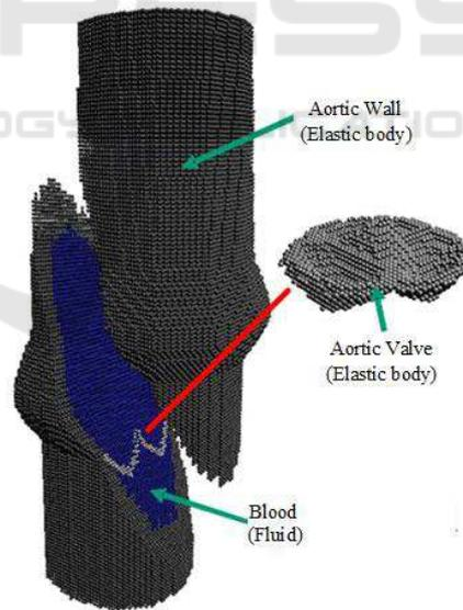
Figure 7: Particle model of the aortic wall and valve.
