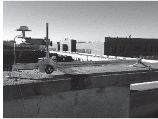
Figure 2: The sledge where the GNSS antenna was mounted.
