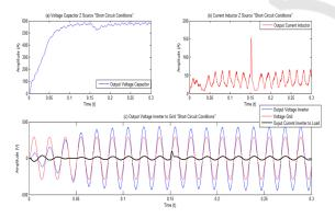
Figure 8: Ouput Waveforms from VZI "Short Circuit Conditions".
