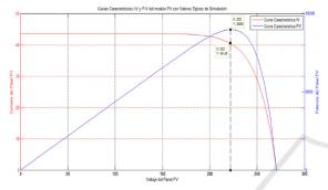
Figure 5: Characteristic curve PV Panel in "STC.
