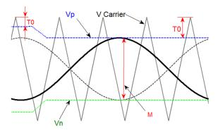
Figure 3: Switching time with "SBC" control method (Zope, 2012).
