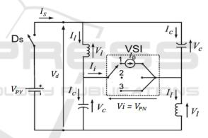
Figure 2: Equivalent circuits of Z Source Inverter (Rajakaruna and Jayawickrama, 2010). (1) Mode 1, (2) Mode 2 and (3) Mode 3.
