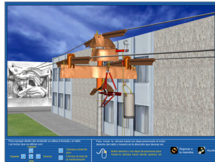
Figure 7: Virtual reality training system for medium tension live line maintenance ALEn 3D MT.
