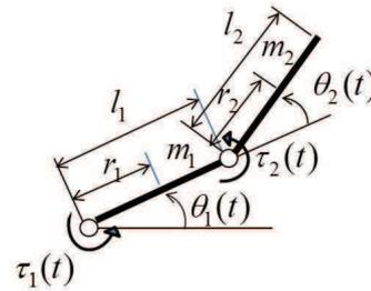
Figure 2: A Model of the 2-Link Manipulator.
