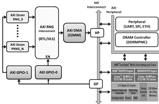
Figure 3: PRNG Platform Based on Zynq.
