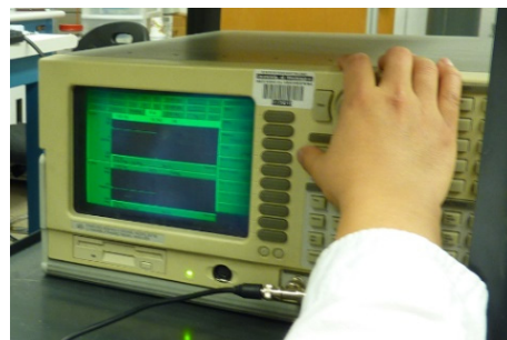
Figure 4: Dynamic signal analyzer used to get the frequency response to obtain the model of the actuator.
