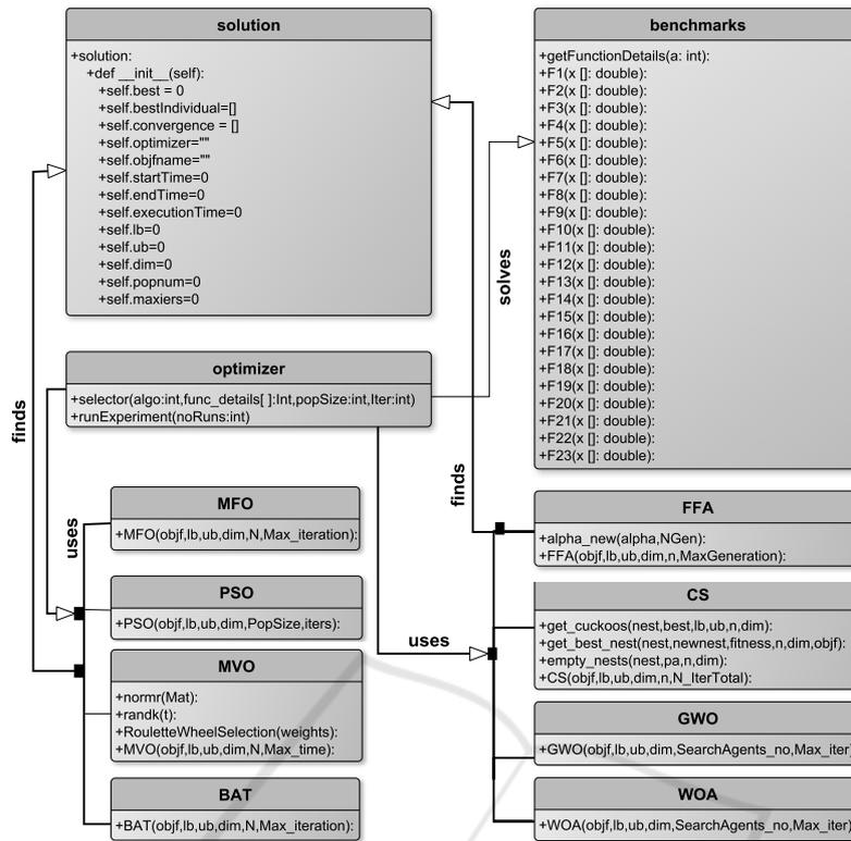
Figure 1: Class diagram of the EvoloPy framework.
