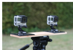
Figure 1: GoPro Hero4 cameras and jig. The distance between the cameras is 0.25 m.
