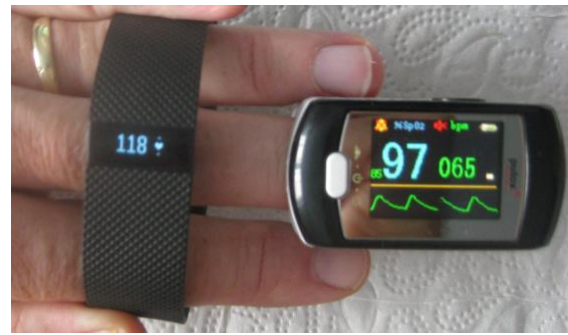
Figure 7: Optical pulse detection is standard in medicine, where monitors like the pulsoxiometers (right device) shine an optical beam through the finger. This yields better contrast than the reflection method of the tested bracelet trackers. Here again, the obtrusive unit (left device) enforces measurement of just any signal, which leads to a totally wrong result of 118 bpm in contradiction to the correct sensing value of 65 bpm.
