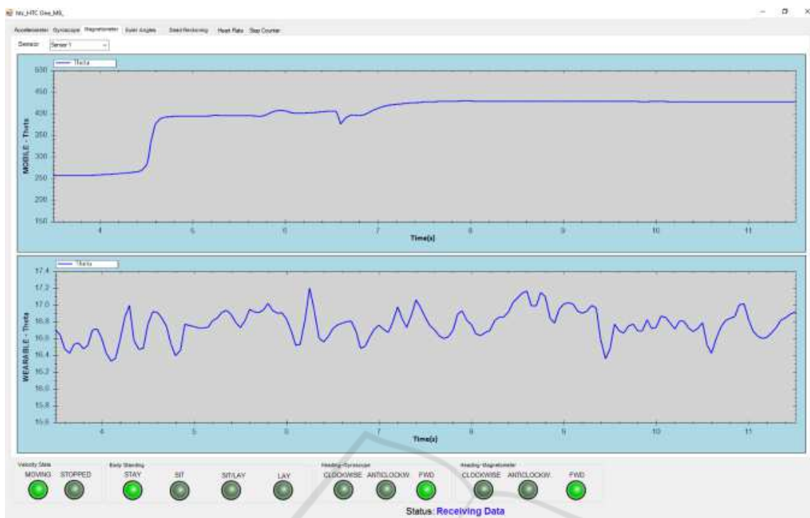
Figure 4: Server Side View, On top the tabs of the graphs view, At the center the data (e.g. magnetometer) of both the phone and smartwatch IMUs, of the given view; bottom-down the state of the person at the current time.
