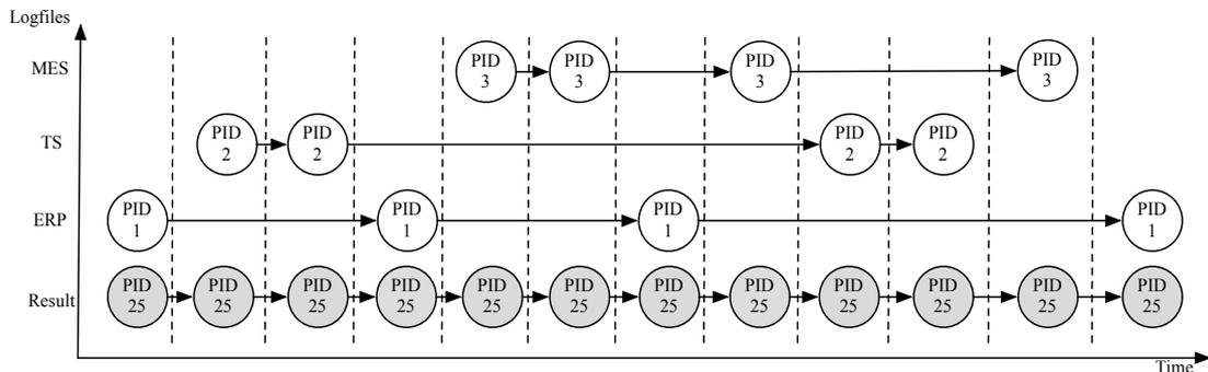
Figure 4: Basic procedure for log file integration (for one process instance).
