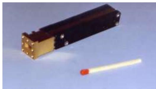
Figure 4: Picture of the 8 mm radiometer (Gorishnyak et al, 2004).
