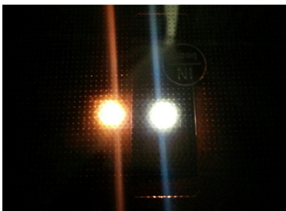
Figure 5: Visualization of a white LED through a ceramic glass: without compensation filter (left) and with compensation filter (right).
