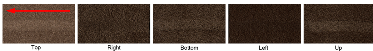
Figure 4: The material sample used for our experiments under different lighting conditions where parts of the sample were brushed into the direction indicated by the red arrow using a finger. Note that the fibers in the unbrushed parts are not arranged straight upwards, which is why there is a larger change in brightness also in these parts.
