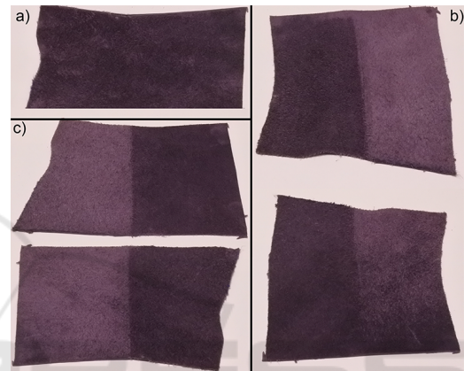
Figure 2: Illustration of the appearance changes due to different fiber orientations: (a) initial state where the fibers are mainly oriented upright, (b) state where the fibers are brushed along and against the dominant fiber orientation defined by the material structure, and (c) state where the fibers are brushed perpendicular to the dominant fiber orientation and along the opposite direction.
