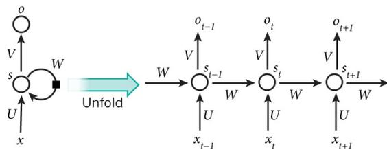
Figure 3: RNN basic structure and unfolding in time according to the number of sequence elements. In this figure, the network is unrolled into a 3-layer NN.
