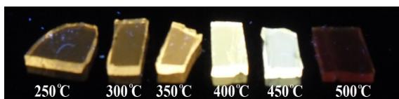
Figure 4: Photo of the PTR glass GS10 samples subjected to the IE and subsequent heat treatment at temperatures 250-500 °C.
