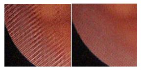
Figure 3: Left- cropped section of original RGB image to illustrate the honey-comb structured artefact caused by the fibre-optic bundle; Right: pre-processed image with artefact suppressed.
