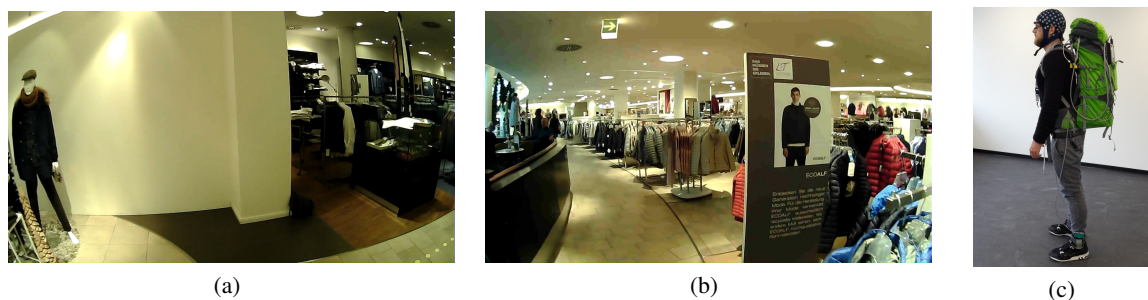
Figure 3: Real World Visual Processing example of one subject. (a) first frame, starting point of the subject; (b) last frame, end point reached; (c) Picture showing the working recording setup using EEG, eyetracking, worldcam and step-sensor.
