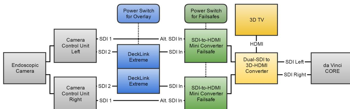
Figure 1: Overview of the setup we use to overlay the video streams of the da Vinci S surgery system with computer graphics including failsafes and a 3D TV. Grey: standard da Vinci S components. Blue: overlay system (video capture cards in a computer). Green: Mini-converters used as loss-of-signal switches. Yellow: 3D HDMI conversion and 3D TV.
