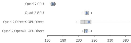
Figure 6: Photon-to-photon latency (in ms) from the endoscopic camera to the surgeon’s display when passing image data through CPU or GPU memory. The DirectX setup dropped some frames and has been purposely cropped in the plot to better show the results of the other setups. The blue “x” marks the average latency.
