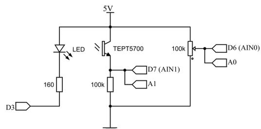
Figure 3: Schematic of the test equipment. The labels are based on Arduino Uno pin mapping. "A0" and "A1" are used during calibration.
