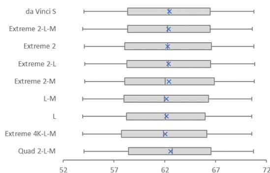
Figure 4: Photon-to-photon latency (in ms) of the da Vinci S surgical system with various configurations of our system. (“L” stands for loss-of-signal switchers; “M” for the MC-100 SDI-to-3D-HDMI converter.) The blue “x” marks the average latency.
