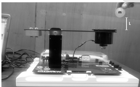
Figure 11: VTOL under external disturbance test.
