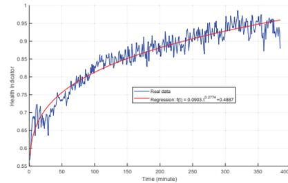
Figure 9: Health indicator for the bearing (6H50).
