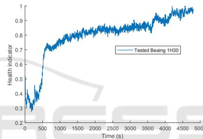
Figure 10: Health indicator for the bearing (90 minutes).
