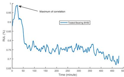
Figure 11: RUL estimation for the tested bearing (6H50).
