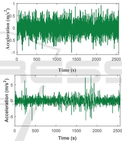
Figure 2: Sensors measurement for normal condition (top) and degradation bearing (bottom).
