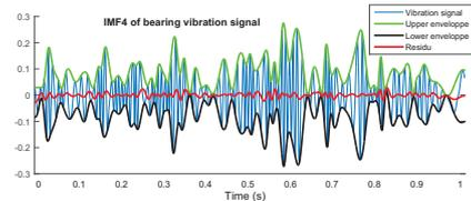
Figure 3: The EMD results of vibration signal.
