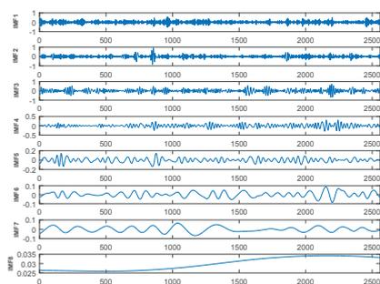
Figure 4: The EMD decomposed results of vibration signal.
