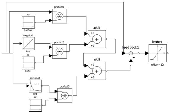
Figure 7: The PID controller, which has three coefficients which are to be optimized in order to provide the right control signals to the regulator.
