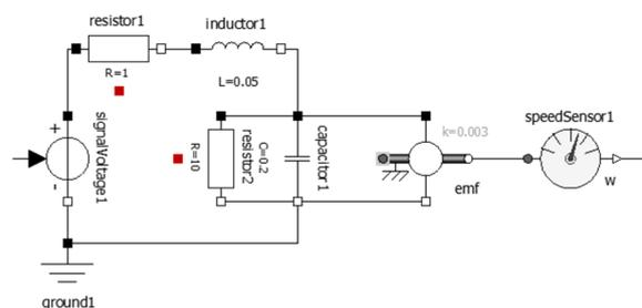
Figure 6: The DC motor, a mechanical system which rotates at a speed defined by its input voltage and measured by a speed sensor.
