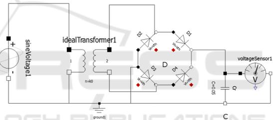
Figure 1: The full wave rectifier. Note the four diodes bridge (D), a capacitor (C), the AC generator on the left and the DC voltage sensor on the right.
