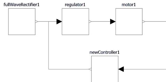
Figure 4: The box diagram of the DC motor controller, which consists of four subsystems, a full-wave rectifier, a voltage regulator, a mechanical DC motor and a PID controller.
