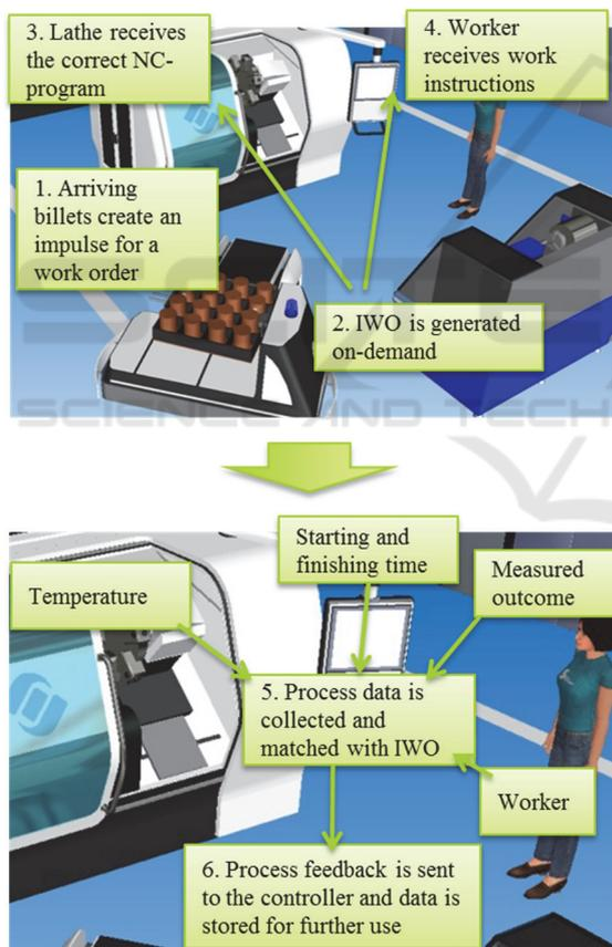
Figure 1: Principle of Intelligent Work Order.
