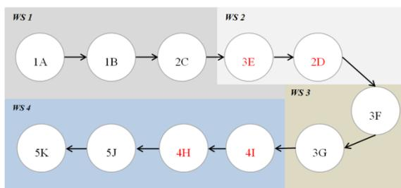
Figure 5 : Presedence diagram of recommendation work station.
