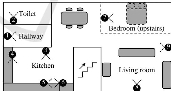
Figure 5: Sensor System; showing the sensor locations.
