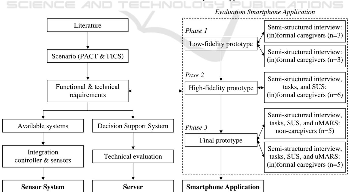
Figure 1: General iterative design process of the HMS.
