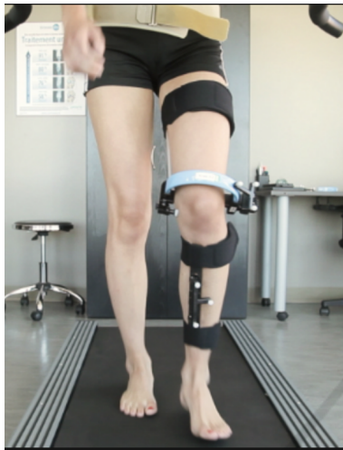
Figure 2: Knee kinematic acquisition system.
