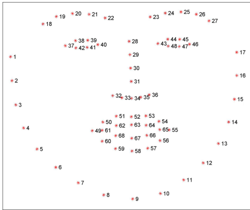
Figure 3: Position of the 68 face landmarks detected. Source: (Sagonas et al., 2013).
