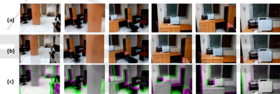
Figure 2: Example for Indoor Alignment. (a) Selected frames from the observed video. (b) The corresponding frames retrieved from the reference video (after temporal alignment). (c) Fusion Image (Red and Blue channels of color image are assigned to the observed frame, while the Green channel is assigned to the reference frame).
