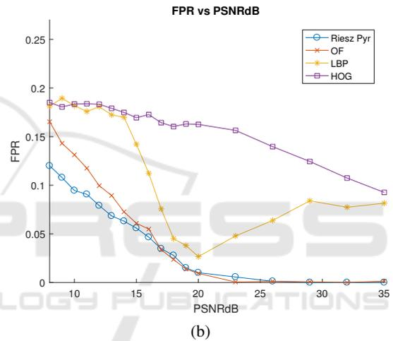
Figure 6: Performance curves of different subtle motion spotting techniques in presence of different levels of Gaussian noise.
