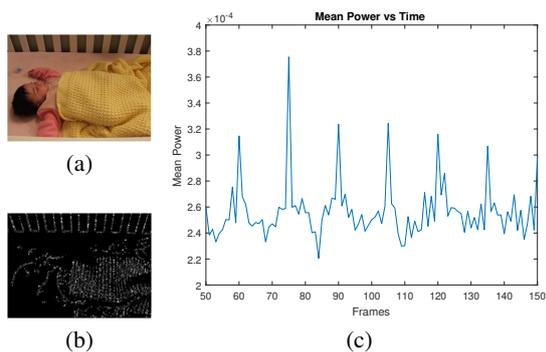
Figure 4: Subtle motion detection for breathing measurement. (a) is the a frame of a video of a baby sleeping, (b) is the masked phase norm and (c) is the obtained signal.
