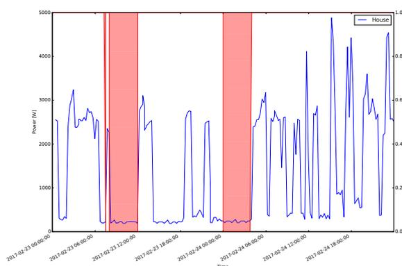
Figure 8: Consumption of one household during 48 hours, with two 4-hour cuts (in red). A really short cut (test) before the first 4-hour cut can also be observed.
