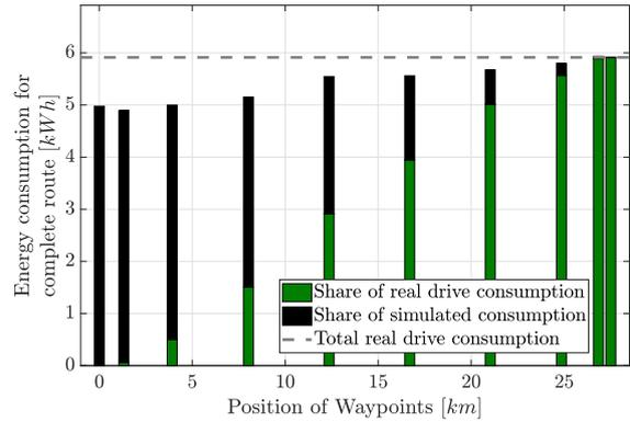
Figure 8: Comparison of predictively determined and real energy consumption. At each waypoint, energy consumption for the entire route is calculated from previous real drive and remaining energy demand estimation.
