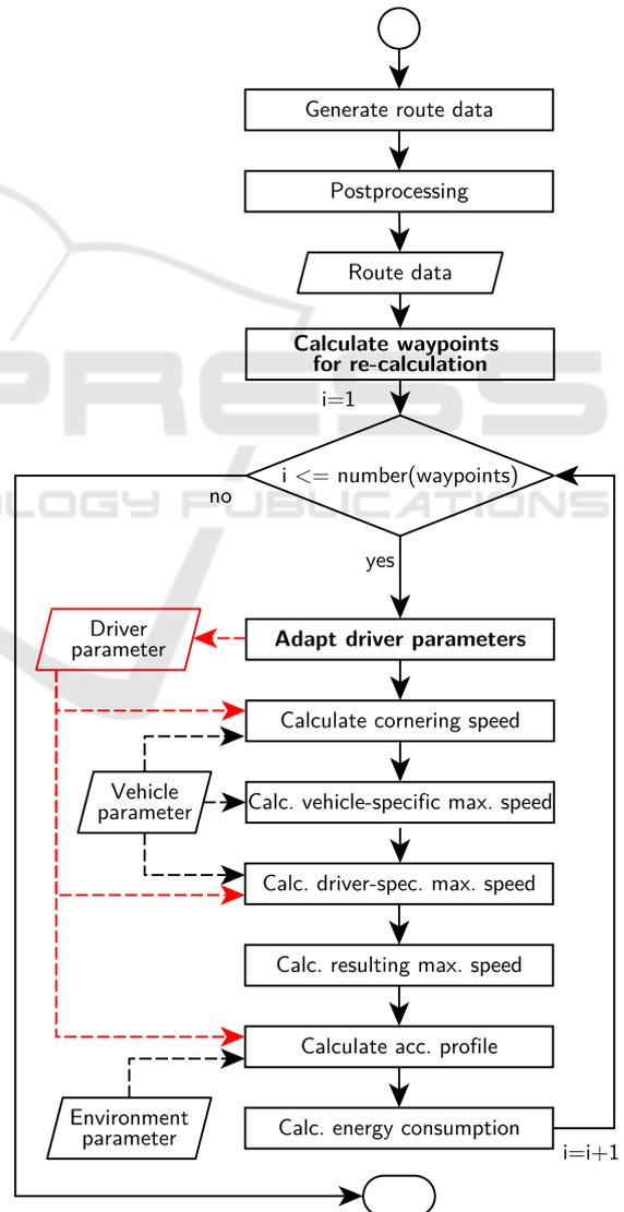
Figure 5: Flowchart of the main algorithm. The red arrow indicates the usage of driver parameters. Bold text indicates a new functions within the framework of our methodology.
