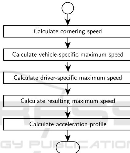
Figure 2: Determination of vehicle motion profile based on algorithm described in (Kruppok et al., 2017).
