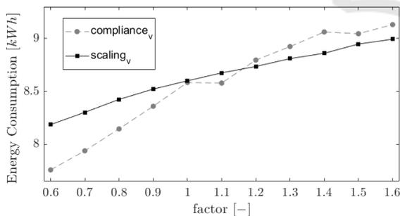
Figure 4: Energy consumption for the variation of the driver parameters  $scaling_a$  and  $compliance_v$  between 0.6 and 1.6 with a step size of 0.1.
