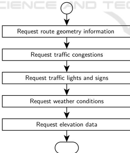
Figure 1: Flow chart of route generating algorithm. The input data are starting point, destination, time and optionally one or more waypoints (Gutenkunst et al., 2015).
