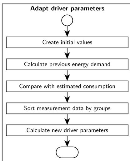
Figure 6: Algorithm for adapting the driver parameters.
