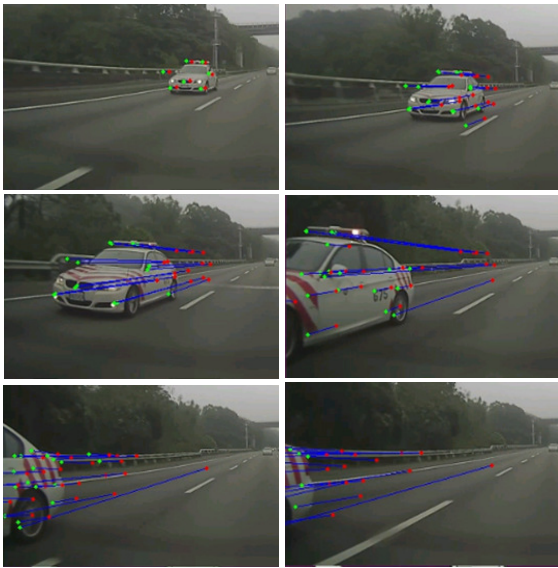
Figure 9: An example result of the overtaking vehicle detection and tracking.
