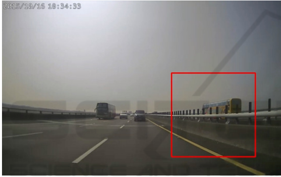
Figure 7: The use of segmentation and CNN at the same time can still be erroneous for repetitive patterns.
