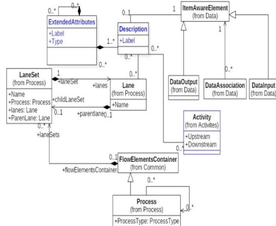
Figure 2: Extract of the used BPMN meta-model.
