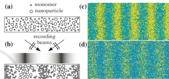
Figure 1: Holographic assembly of nanoparticles in an NPC material (a) before and (b) after holographic exposure. EPMA images of (c) Si (nanoparticles) and (d) S (the formed polymer) atomic density distributions after holographic exposure.
