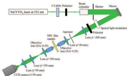
Figure 2: Setup for coaxial holographic digital data page recording.
