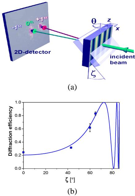
Figure 7: (a) Recording dynamics of the diffraction efficiency probed by a 633-nm laser beam at a recording intensity of  $75 \text{ mW/cm}^2$ . (a) Schematic of the slow-neutron beam diffraction via an NPC transmission grating. (b) Peak (Bragg-matched) diffraction efficiencies  $\eta_p$  as a function of NPC grating's tilt angle  $\zeta$  for an incident very cold neutron beam at a neutron wavelength of 3.76 nm, while the solid curve is a theoretical plot (Klepp et al., 2011).
