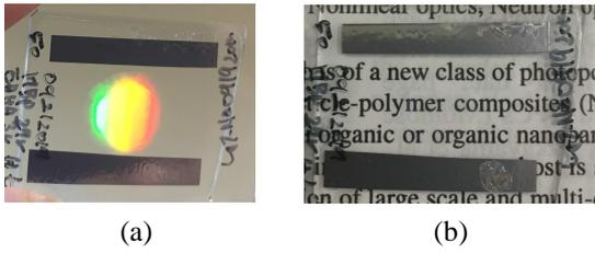
Figure 5: (a) Photograph of an NPC volume grating under white light illumination from a fluorescent lamp. (b) Photograph of the same grating viewed from the top.
