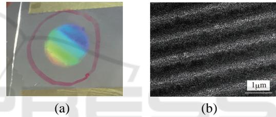
Figure 8: (a) A photograph of an NPC transmission plane-wave grating at grating spacing of  $1 \mu\text{m}$  under white light illumination from a fluorescent lamp. (b) A transmission-electron microscope image of the cross section of the grating.
