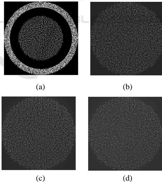
Figure 3: (a) Digital data page pattern with the 9:16 symbol modulation code. (b) Magnified image of the straight-through image via a uniformly cured thiol-ene based NPC film. (c) Magnified image of the reconstructed digital data page pattern from a recorded thiol-ene based NPC film. (d) Magnified image of the reconstructed digital data page pattern from a recorded thiol-yne based NPC film.
