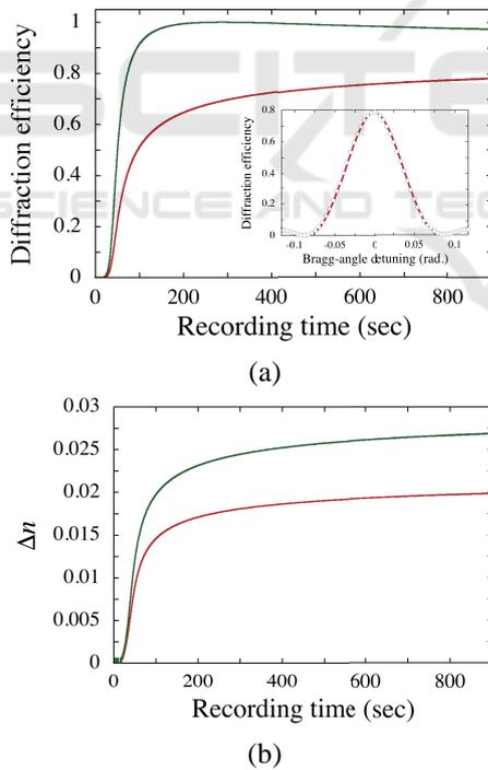
Figure 6: (a) Recording dynamics of the diffraction efficiency probed by a 633-nm laser beam at a recording intensity of  $75 \text{ mW/cm}^2$ . The curve in green is the extrapolated recording dynamics of the diffraction efficiency at 532 nm as described in the text. The inset is a Bragg-angle detuning dependence of the diffraction efficiency probed at 633 nm. (b) Buildup dynamics of  $\Delta n$  at wavelengths of 532 nm (green) and 633 nm (red).
