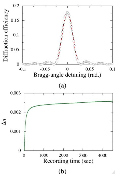
Figure 9: (a) Bragg-angle detuning dependence of the diffraction efficiency at 633 nm. (b) Buildup dynamics of  $\Delta n$  at wavelengths of 532 nm.
