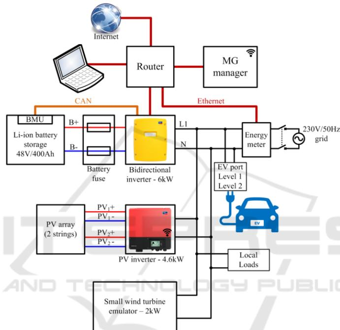
Figure 5: Diagram of the smart Residential MG designed as an EV charging station.
