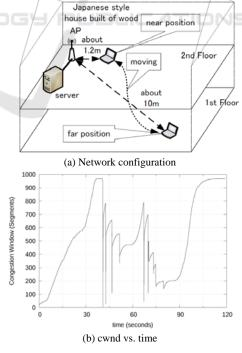
Figure 3: TCP data transfer over 802.11n WLAN. (Nomoto et al., 2014).
