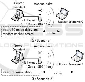
Figure 6: Experimental configuration.
