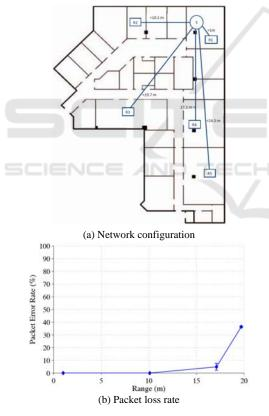
Figure 2: UDP data transfer over 802.11ac WLAN. (Dianu et al., 2014).
