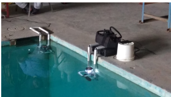
Figure 4: Aquatic Test. Both the transmitting and receiving nodes during an aquatic range test are shown. The emitter appears as a constant (but dim) light. Here the receiver is not transmitting.
