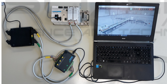
Figure 4: Experimental platform with M340 PLC, FACTORY I/O and USB DAQ Advantech 4750.
