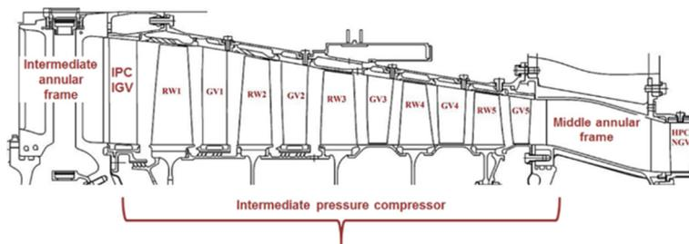
Figure 2: The diagram of investigated compressor flow path.
