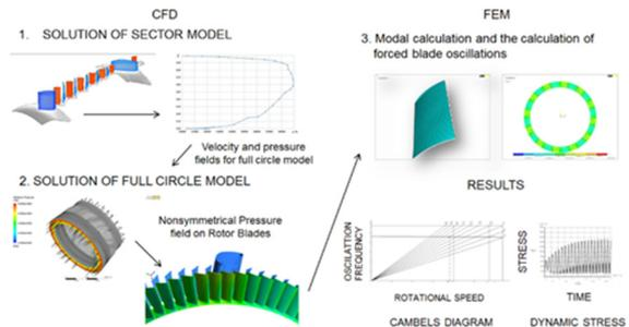
Figure 5: Scheme of method for calculation compressor rotor blades forced oscillations.
