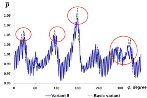
Figure 11: Graphs of relative static pressure variation for basic compressor variant and variant 9.
