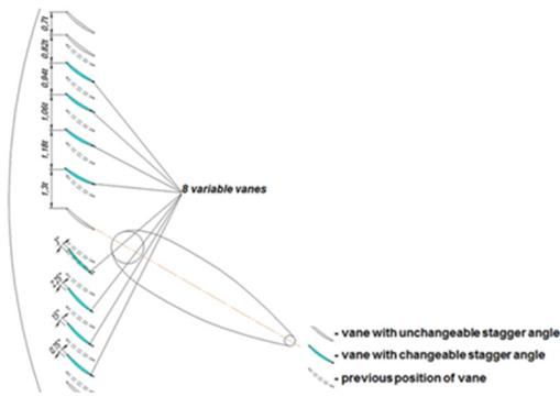
Figure 9: The diagram of GV blades rotation.
