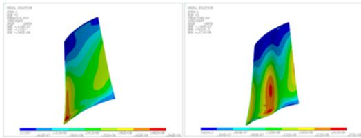
Figure 7: Equivalent stresses at the resonance in RW5 blade (original is on the left, Shvarov's profile is on the right).
