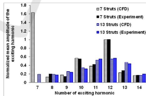
Figure 12: Comparison of excitation amplitudes of harmonics of the basic 7-struts and 13-struts annular frame obtained in experiment and CFD calculation.
