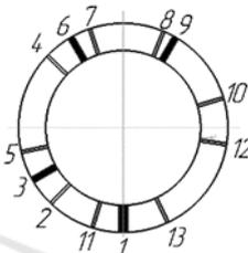
Figure 14: Optimized 13-struts annular frame.
