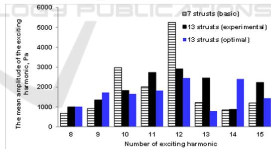
Figure 15: Comparison of exciting harmonics amplitudes of the original 7-struts, 13-struts frame by JSC "Kuznetsov" and optimized 13-struts annular frame.
