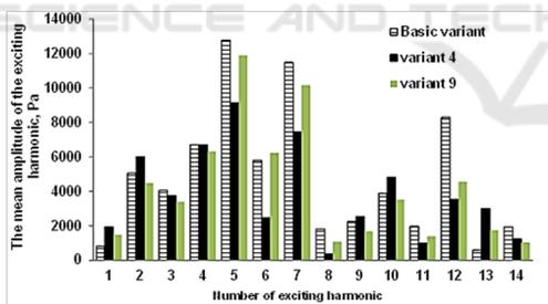
Figure 10: The mean of exciting harmonics amplitudes acting on RW5.
