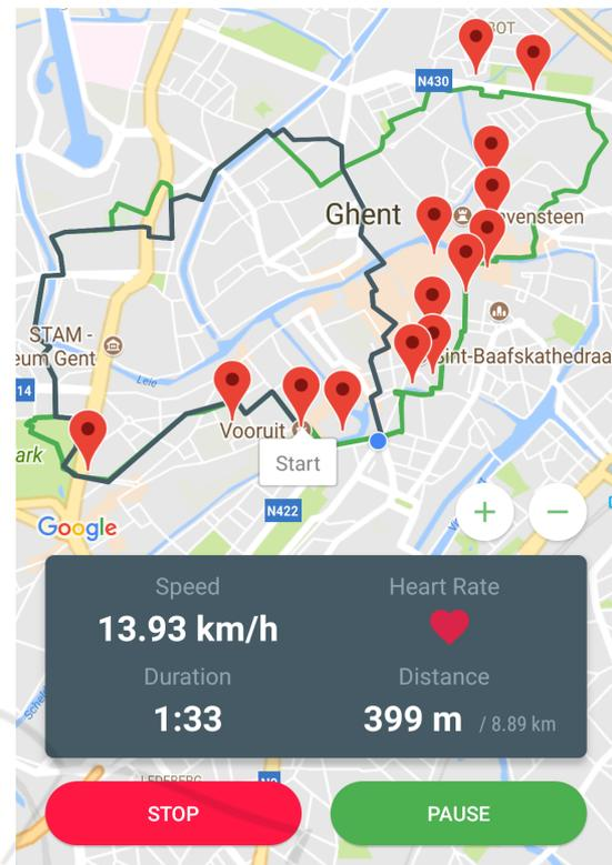
Figure 2: *Runamic: A Dynamic Route Generation Application.* The figure shows an active running screen of the application. The green line segment in the figure denotes the currently followed running route while the blue one denotes a shorter route, requested dynamically during the run.
