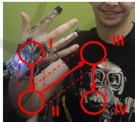
Figure 3: The wearable glove system with the dynamic gesture graph in the form of letter "N".
