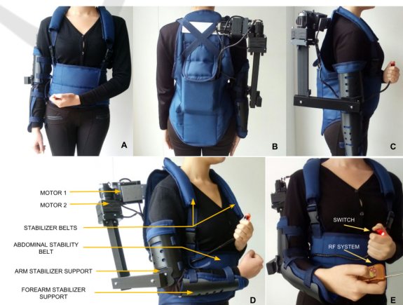
Figure 5: Prototype of shoulder rehabilitation robot system. (A) front and (B)posterior sagittal axis of the device placed on patient. (C) Right view. (D) Stabilizing components. (E) Control accessories.
