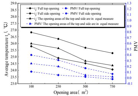
Figure 8: The average temperature and PMV of the second floor personnel activity area.
