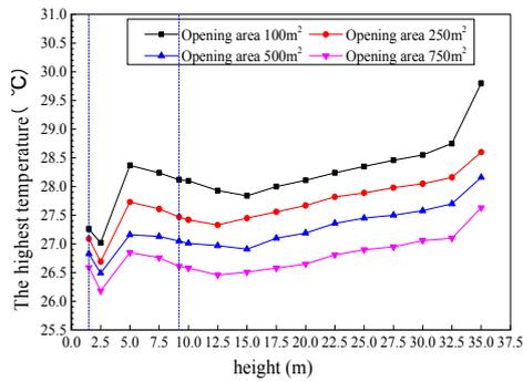
Figure 5: The highest temperature of full side opening condition.
