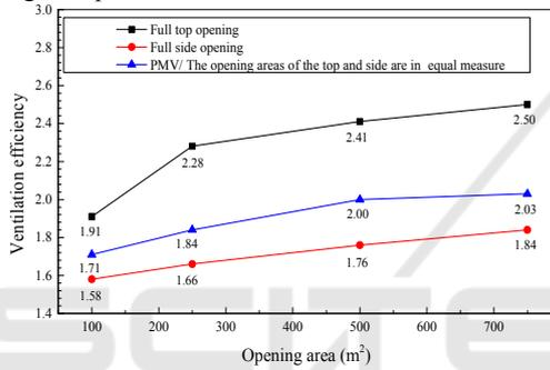
Figure 9: Natural ventilation efficiency of each condition.
