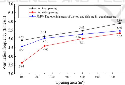
Figure 10: Natural ventilation frequency of each condition.
