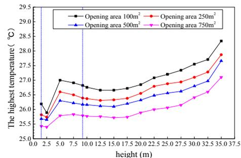
Figure 4: The highest temperature of full top opening condition.
