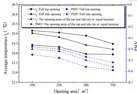
Figure 7: The average temperature and PMV of the first floor personnel activity area.
