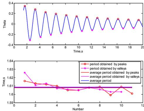
Figure 5: Slushing frequency when FP=0.5, LA=0.6 g
