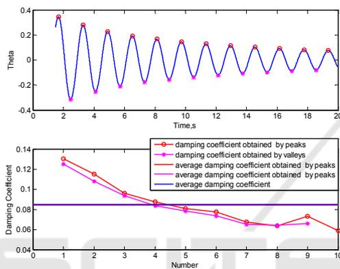
Figure 6: Slushing damping when FP=0.5, LA=0.6 g
