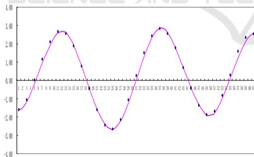
Figure 3: The tidal elevation comparison (point: observation; line: model outputs).
