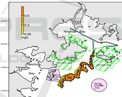
Figure 6d: Influence scope after oil spill over 48 h at ebb tide moments under northeast conditions.
