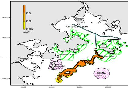
Figure 6a: Influence scope after oil spill over 48 h at high tide moments under northeast conditions.
