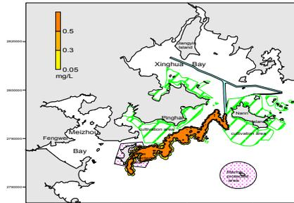
Figure 6b: Influence scope after oil spill over 48 h at flood tide moments under northeast conditions.
