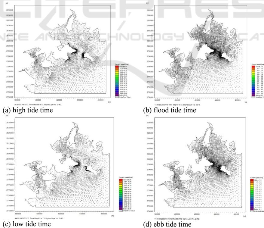
Figure 5: The simulated surface water currents near Nanri Island at different times.
