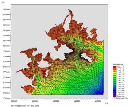
Figure 2: The grid configuration and the bathymetry of the simulated area.
