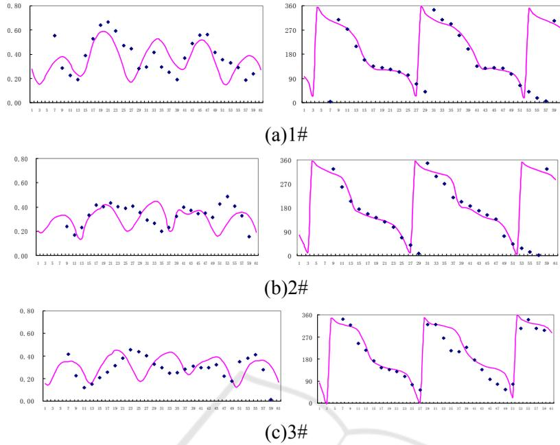
Figure 4: The current velocities (left) and direction (right) comparison form the model and observations at different station (point: observation; line: model outputs).
