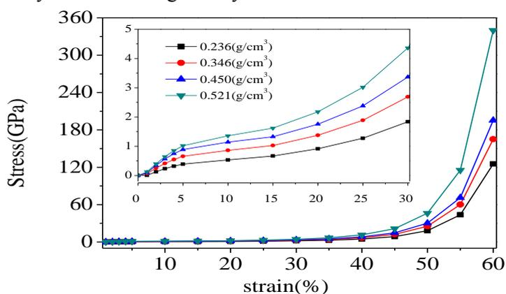
**Figure 9.** Stress-strain curve of composite aerogel with different densities during compression.
