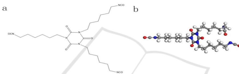
**Figure 1.** The model of tri-isocyanate Desmodur N3300: (a) molecular structure, (b) ball stick model.
