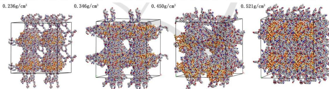
**Figure 5 .** Structural model of polymer cross-linked aerogels at four different densities
