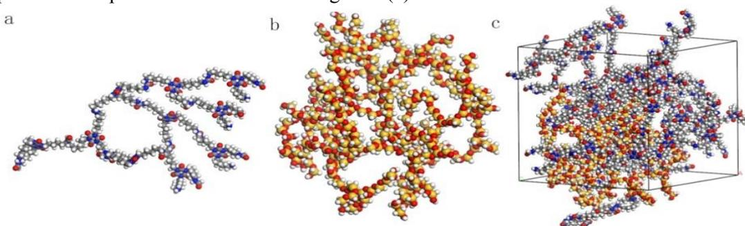
**Figure 2.** Structure models: (a) N3300 polymer, (b) the nanoparticle of silica aerogel and (c) the cell of composite aerogel
