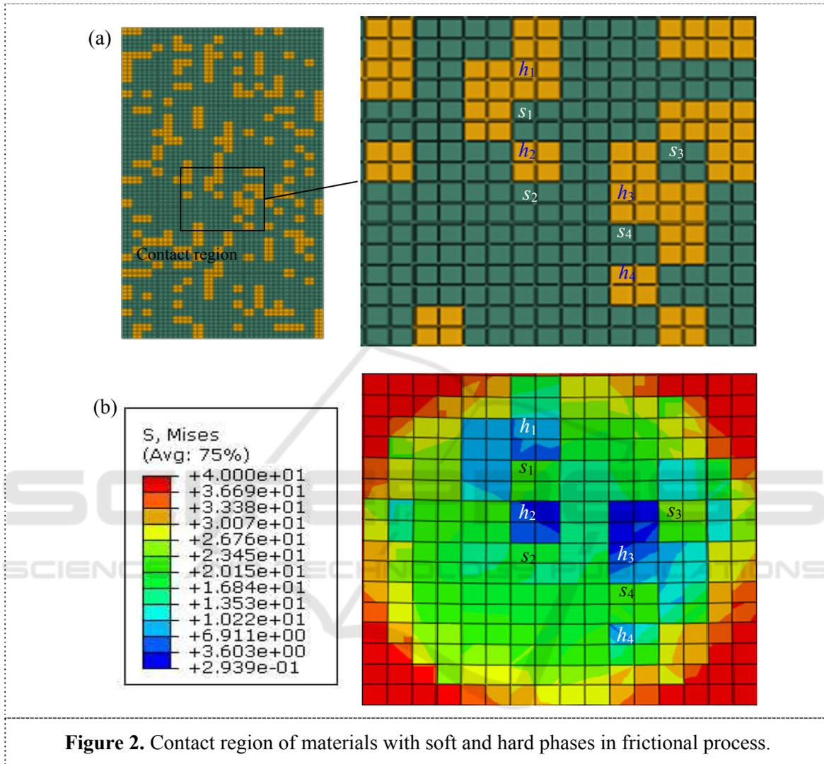
Figure 2. Contact region of materials with soft and hard phases in frictional process.
